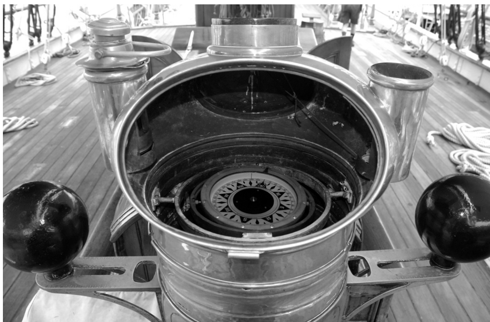
ELISSA's binnacle and compass. This is the view that her helmsman worked with. Her courses are now called out in the 360 degree scale marked on the card, but the diamond markings of an older system are easier for the helmsman to read by the dim lights of the candles mounted in the tubes seen at each side.
